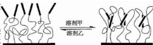
图 4 嵌段共聚物在不同溶剂作用下的构象重排 Figure 4 Amphiphilic block polymer brush images different morphology when treated with different solvents
